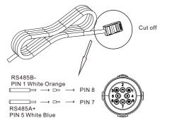
g.The standard RS485 cable length is 15m.If need longer RS485 cable, please use an ethernet coupler to extend and make sure RS485 cable less than 100m(the recommended length is less than 25m).
