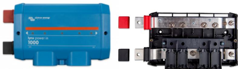
The lynx power in module is used to connect batteries via an external fuse. It can be useful if you have multiple parallel strings. Due to the extremely high short circuit current potential of most battery banks, it is suggested to use an external fuse system with an appropriate fault current interruption rating (such as an NH HRC).
