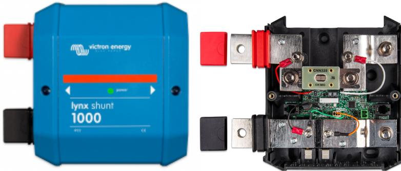
The Lynx shunt contains a positive bus-bar with space to mount a CNN fuse and a negative bus-bar with a shunt. It also contains battery monitoring electronics. The Lynx shunt can send via the VE.CAN bus battery monitoring information to a CCGX or VGX or to a third party CANbus monitoring system, such as a NMEA2000. The CCGX, VGX or third party display acts as battery monitor display and is also used to set up the built-in battery monitor.
