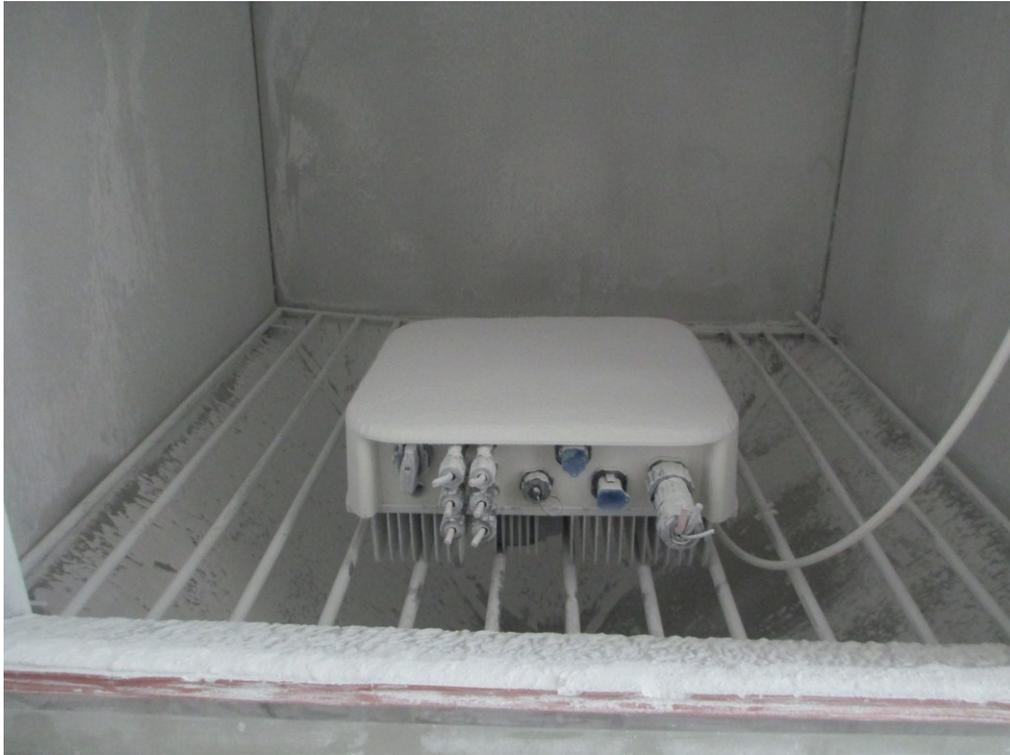
Test setup of IP6X
