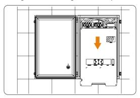
Figure 7-90 Removing the plate
