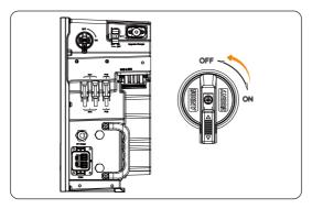
Figure 12-2 Turning off the DC switch
