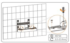
Figure 6-36 Securing the base
