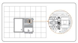
Figure 7-92 Installing the Wi-BR
