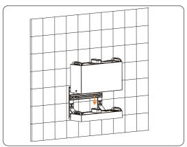
Figure 6-37 Placing battery module
