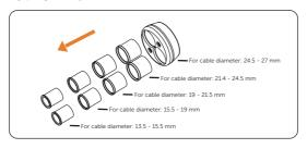
Figure 7-24 Taking out sealing plug
