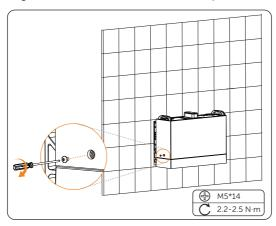
Figure 6-38 Tightening screws
