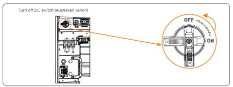
Figure 8-7 Turning off DC switch
