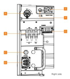
Figure 2-14 Ports of an inverter
