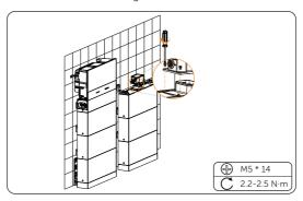
Figure 6-30 Placing the series box
