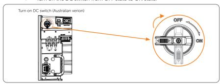
Figure 8-6 Turning on DC switch
