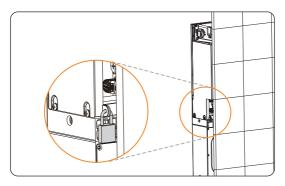
Figure 7-74 Installing the padlock
