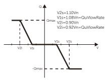
Figure 9-60 Curve Q=f(V)
