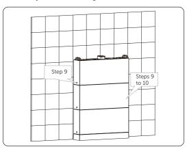
Figure 6-14 Placing battery modules
