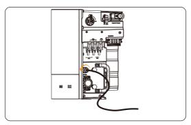
Figure 12-15 Disconnecting the CT/Meter cable
