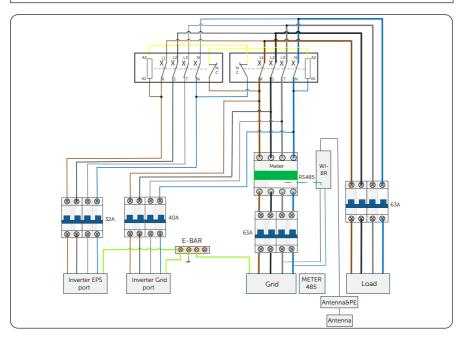
Figure 7-95 Matebox wiring diagram (with Wi-BR)
