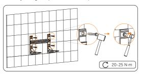
Figure 6-35 Tightening expansion screws
