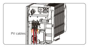
Figure 7-44 Connecting PV cables
