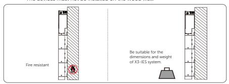
Figure 4-5 Installation carrier requirement
