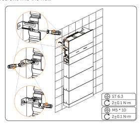
Figure 6-53 Locking the inverter brackets
