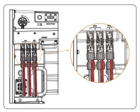
Figure 7-35 Well connected PV cables
