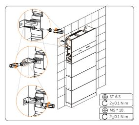
Figure 6-28 Locking the inverter brackets
