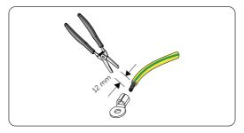
Figure 7-113 Stripping the PE cable
