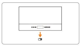
Figure 6-25 Removing the dustproof cover
