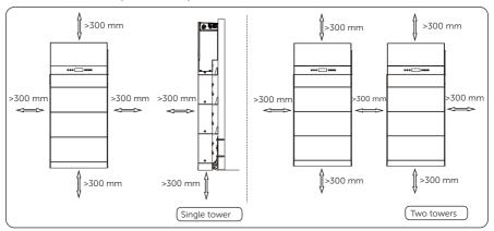
Figure 4-6 Clearance requirement
