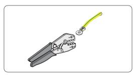
Figure 7-114 Crimping the PE cable
