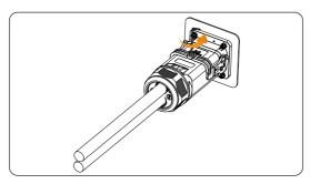
Figure 12-10 Loosening the AC connector
