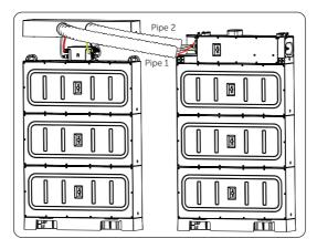
Figure 7-11 Inserting pipes into the cover
