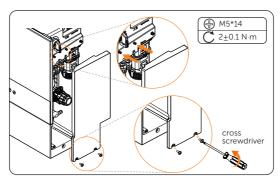
Figure 7-70 Locking the cable shielding board
