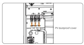
Figure 7-43 Removing the dustproof cover
