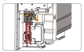
Figure 12-8 Pulling out PV dustproof buckles
