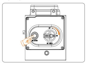
Figure 8-3 Turning on the battery
