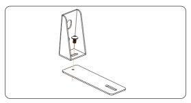
Figure 6-7 Attaching two brackets
