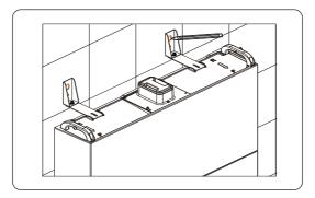
Figure 6-16 Marking the position of BMS
