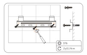
Figure 6-59 Securing the bracket
