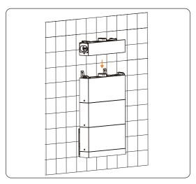
Figure 6-47 Placing the BMS
