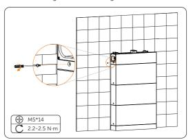
Figure 6-23 Tightening M5 screws
