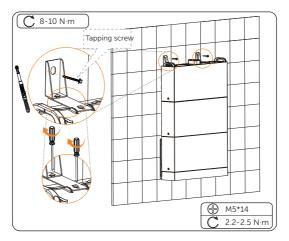
Figure 6-46 Securing the assembled bracket
