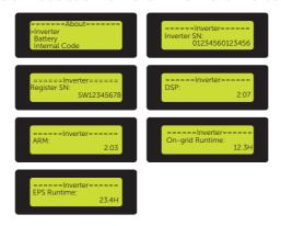
Figure 9-103 Displaying the inverter information
