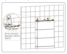
Figure 6-21 Tightening the BMS brackets
