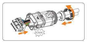
Figure 7-28 Wiring the AC connector
