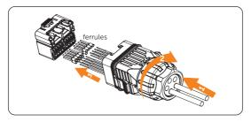
Figure 7-59 Inserting wires into ferrules
