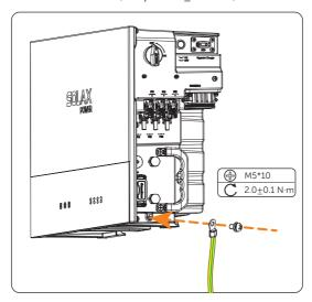
Figure 7-18 Securing the PE cable
