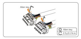
Figure 7-27 Locking wires in the AC connector
