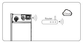
Figure 7-75 WiFi mode connection diagram
