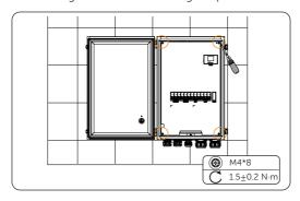
Figure 7-139 Securing the plate
