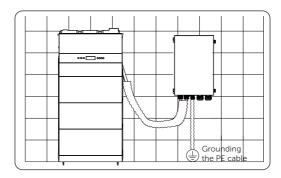
Figure 7-119 Connecting the PE cable to ground
