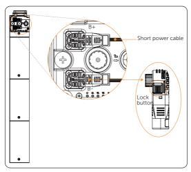
Figure 7-6 Removing short power cable
