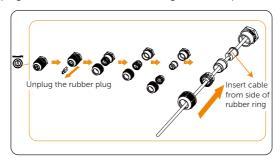
Figure 7-93 Threading the Wi-BR cable through Antenna&PE port
