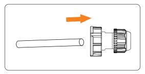
Figure 7-64 Threading the communication cable
