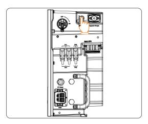
Figure 8-4 Pressing the inverter button
