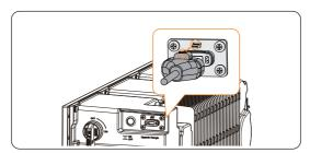
Figure 7-82 Installing the WiFi connecting cable
