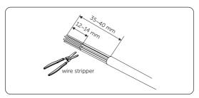
Figure 7-58 Stripping cables
