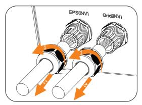
Figure 12-19 Disassembling EPS(INV) and Grid(INV) cables
