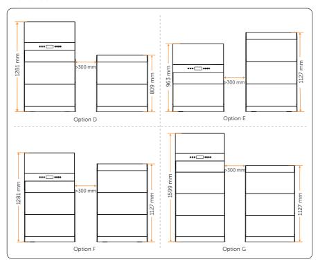
Figure 4-4 Installation options for two towers
