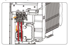
Figure 12-7 Pulling out PV connectors
