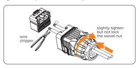
Figure 7-56 Stripping cables
