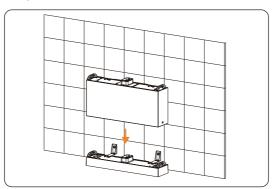
Figure 6-12 Placing the battery module
