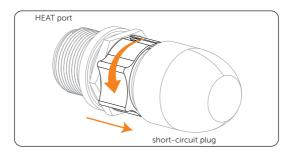
Figure 7-8 Closing short-circuit plug
