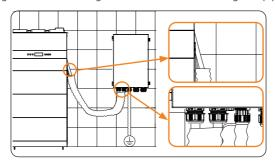
Figure 7-123 Well connected meter cable
