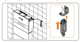
Figure 7-84 Plugging the dongle
