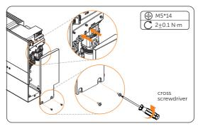
Figure 7-72 Locking the cable shielding board
