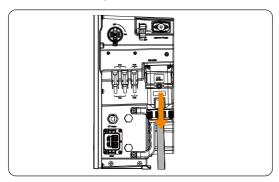
Figure 12-12 Unplugging the AC connector
