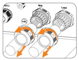
Figure 12-20 Disassembling Grid and Load cables
