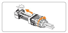
Figure 7-61 Inserting the terminal block into the connector
