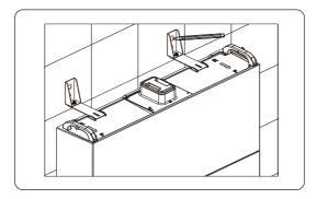
Figure 6-41 Marking the position of BMS
