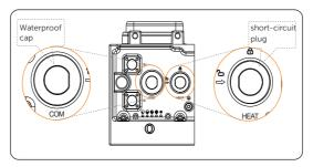
Figure 7-7 Removing waterproof cap
