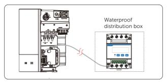
Figure 14-8 Connecting inverter to meter
