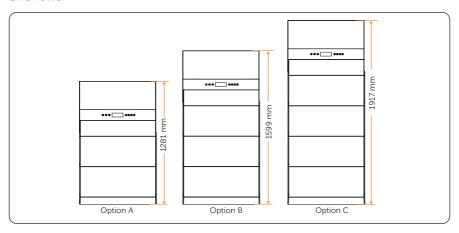
Figure 4-3 Installation options for one tower
