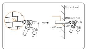
Figure 6-9 Drilling holes
