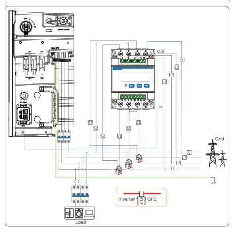
Figure 14-10 System wiring with CT-connected meter
