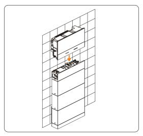
Figure 6-26 Installing the inverter
