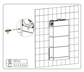
Figure 6-48 Tightening M5 screws
