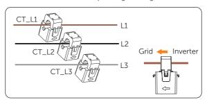
Figure 14-2 Clipping CTs to grid cables
