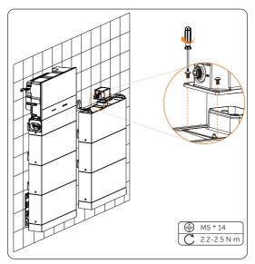
Figure 6-55 Placing the series box
