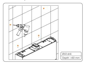
Figure 6-44 Drilling holes
