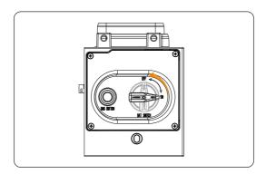
Figure 12-3 Turning off the BAT switch
