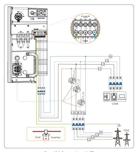
Figure 14-1 System wiring with CT
