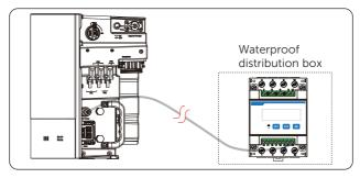
Figure 14-13 Connecting inverter to meter
