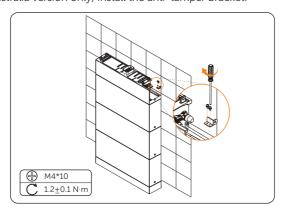
Figure 6-49 Install the anti-tamper bracket
