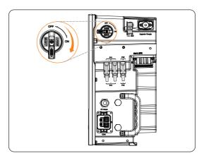
Figure 8-2 Turning on the DC switch
