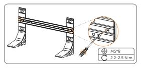
Figure 6-32 Attaching base support and transverse plate
