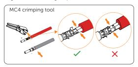
Figure 7-38 Crimping cables with PV pin contacts
