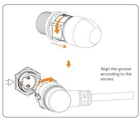
Figure 7-12 Locking heater cable
