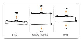
Figure 6-31 Removing dust covers
