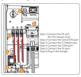
Figure 7-14 Wiring sequence of the inverter
