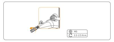
Figure 12-18 Disconnecting grounding cable
