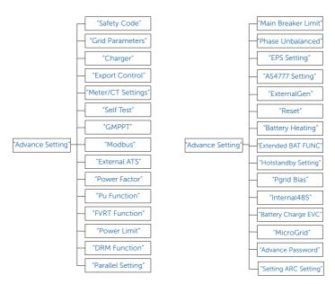
Figure 9-7 Advance setting diagram
