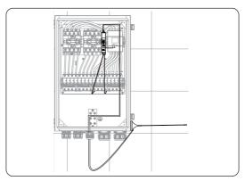
Figure 7-99 Connecting the Wi-BR and antenna
