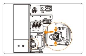
Figure 12-14 Disconnecting the communication connector
