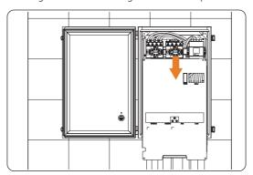
Figure 7-88 Removing the plate
