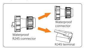
Figure 7-63 Disassembling the waterproof RJ45 connector
