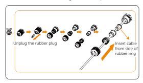
Figure 7-98 Threading the Wi-BR cable through Antenna&PE port
