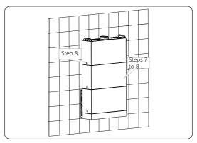
Figure 6-39 Placing battery modules
