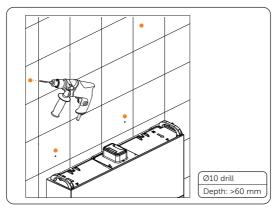
Figure 6-19 Drilling holes
