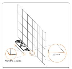
Figure 6-6 Placing the base
