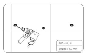
Figure 6-57 Drilling holes
