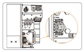
Figure 7-54 Well connected COM port
