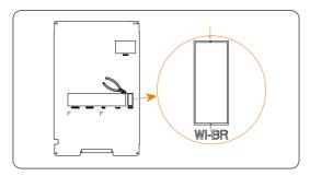
Figure 7-96 Cutting the baffle
