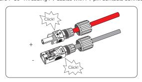
Figure 7-40 Securing PV cables
