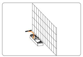
Figure 6-4 Determining whether the base is level
