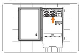
Figure 7-136 Reinstalling the plate
