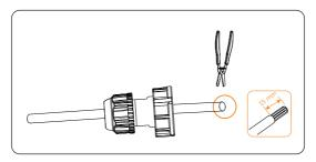
Figure 7-67 Stripping the communication cable for meter
