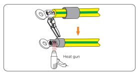
Figure 7-17 Crimping the cable
