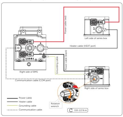
Figure 7-9 Connecting cables
