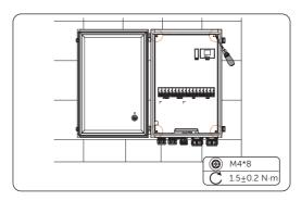
Figure 7-137 Securing the plate
