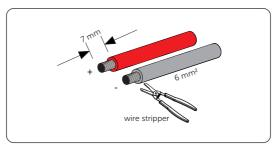
Figure 7-36 Stripping PV cables
