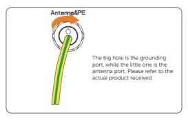
Figure 7-116 Tighting the waterproof connector
