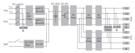
Figure 2-23 X3-IES system circuit diagram
