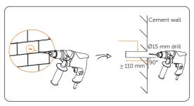
Figure 6-34 Drilling holes
