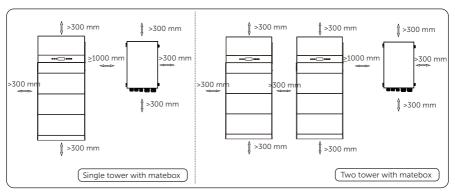
Figure 4-7 Clearance requirement with matebox
