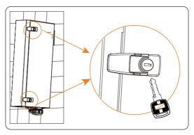
Figure 7-86 Unlocking the buckles
