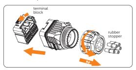
Figure 7-55 Disassembling the communication connector
