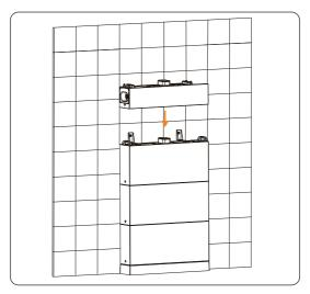
Figure 6-22 Placing the BMS
