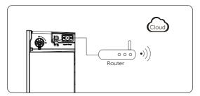
Figure 7-76 LAN mode connection diagram
