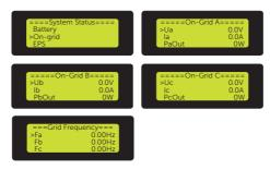
Figure 9-16 Displaying on-grid status
