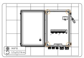
Figure 7-89 Loosening screws on the plate
