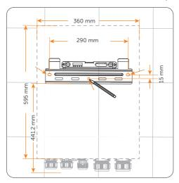
Figure 6-56 Positioning the matebox bracket
