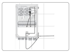
Figure 7-94 Connecting the Wi-BR and antenna
