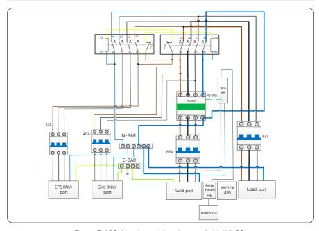
Figure 7-100 Matebox wiring diagram (with Wi-BR)
