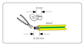
Figure 7-15 Striping the PE cable
