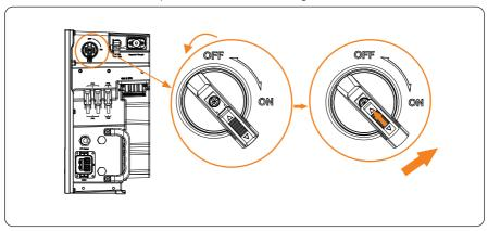
Figure 8-8 Locking DC switch
