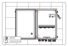
Figure 7-87 Loosening screws on the plate
