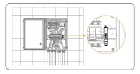
Figure 7-97 Installing the Wi-BR
