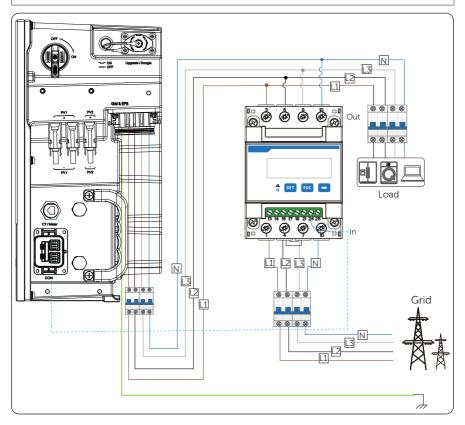
Figure 14-5 System wiring with direct-connected meter
