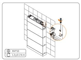
Figure 6-24 Install the anti-tamper bracket
