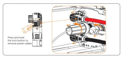
Figure 12-17 Disconnecting battery connectors
