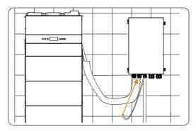
Figure 7-122 Inserting meter cable into the corrugated pipe
