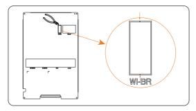
Figure 7-91 Cutting the baffle
