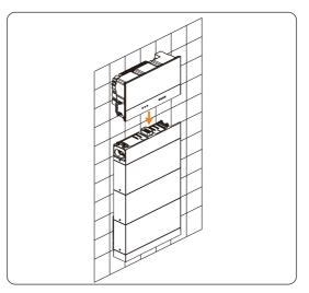
Figure 6-51 Installing the inverter
