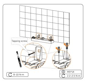
Figure 6-11 Securing the assembled bracket
