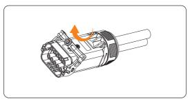
Figure 7-29 Pulling up the latch
