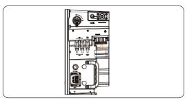
Figure 7-30 Removing the dustproof cover
