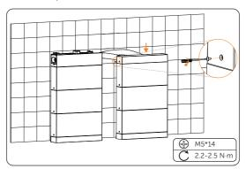
Figure 7-13 Tightening M5 screws
