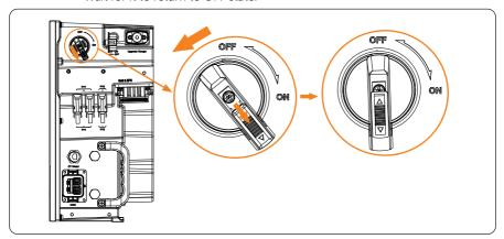
Figure 8-9 Unlocking DC switch
