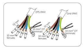
Figure 7-102 Stripping cables and inserting terminals into cables
