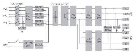
Figure 2-24 X3-IES-P system circuit diagram
