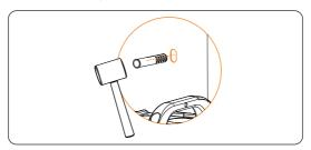
Figure 6-10 Inserting the expansion bolt
