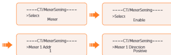
Figure 14-19 Setting meter for the inverter
