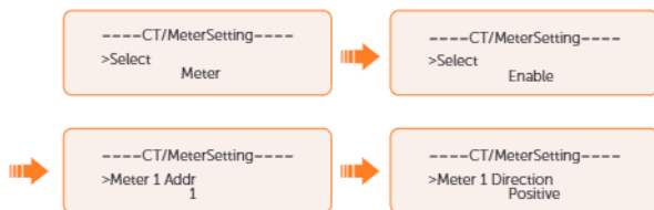
Figure 14-24 Setting meter for the inverter
