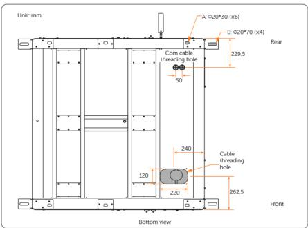
• Secure the cabinet to the foundation through hole A or B.
