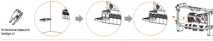
6.6 Finally, use a philips screwdriver to install the baffle back, install the upper cover, and then lock the buckle with a key
