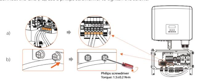
2) Grid(L/N/PE) /Load(L/N) side connection.
