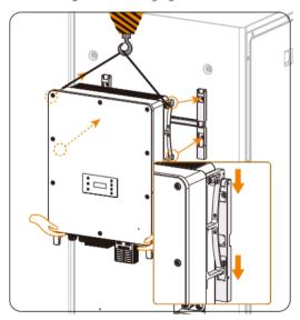
Figure 7-18 Hooking the inverter on the bracket
