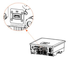
Step 2. Plug Wifi Dongle into the DONGLE port.
