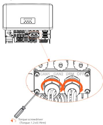
Step 7: Here below are the well connected communication cables.
