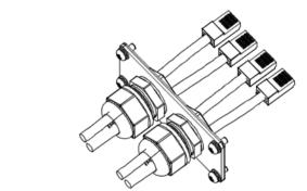
**Step 5.** Insert well crimped CAN1/ CAN2/ DRM/ OFF cables into the corresponding port of the inverter.
