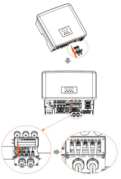
**Step 6.** Tighten the screws and lock the cover on the inverter. And then tighten the swivel nuts.
