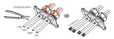
**Step 4.** Crimp each stripped cables with a RJ45 terminal in accordance with CAN1/CAN2/DRM/OFF pin definition.
