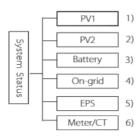
System status contains six content: PV1/PV2/Battery/On-grid (energy feed into or buy from the grid)and EPS(Off-grid) and so on. Press up and down to select, press "Enter" to confirm the selection, and press "ESC" to return to the menu.
