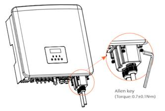
Step 6. Tighten the waterproof fastening head.
