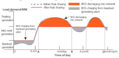
The D-A period is the battery charging period during which discharging is not allowed and the PV will charge the battery first for peak shaving. The ChargeFromGrid" setting determines whether or not to charge from the grid. When "ChargeFromGrid" is set to "Disable", the battery cannot charge from the grid; when "ChargeFromGrid" is set to "Enable" and the actual battery SOC is less than "Max\_SOC", the battery will charge from the grid at no more than "ChargePowerLimits" power.
