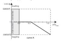
\*) If the grid-connected power of the inverter ≤4.6kW, the Power Factor is 0.95 at 1.0 power; if the grid-connected power of the inverter > 4.6kW, the Power Factor is 0.90 at 1.0 power.
