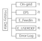
The history data contains five pieces of information: on-grid power of the inverter, EPS power generation, power of the meter /CT and error Error logs.
