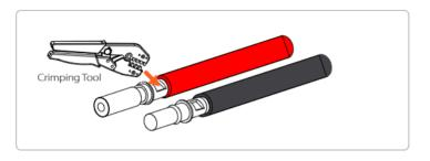
**Step 5.** The battery connectors are divided into 2 parts - the plug and the fastening head. Insert the cable through the fastening head and the opposite plug.
