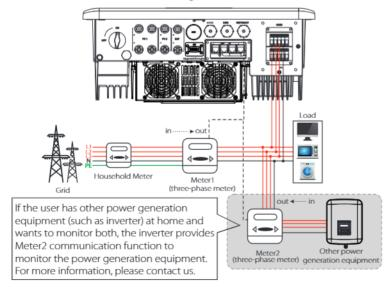
Note: If you want to connect the meter, please ground the GND terminal of the Meter1.
