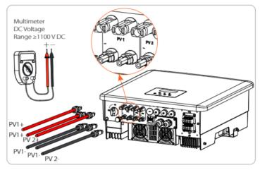
Schematic diagram of the inverter PV connected.
