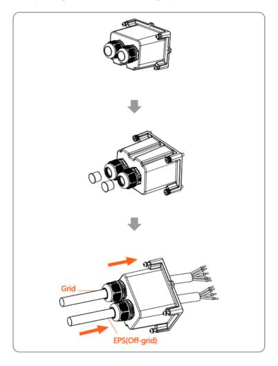
**Step 3.** Remove the 12mm insulation layer at the end of the cable. Insert the ferrules respectively, and make sure that the stripped ends are inserted into the ferrules, and finally use crimping pliers to press tightly.
