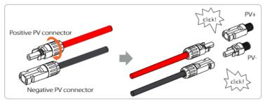
The following is the location of the inverter's positive and negative (PV-/PV+) ports.
