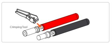
**Step 5.** The PV connectors are divided into 2 parts - the plug and the fastening head. Insert the cable through the fastening head and the opposite plug. Note that the red and black lines correspond to different of plugs. Finally, force the cable pair into the plug, will a "click" sound , which indicates that the connection is complete.
