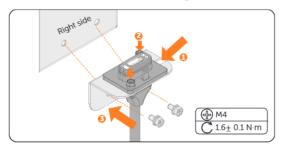
Figure 15-35 Installing the WiFi stand
