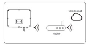
Figure 8-66 Wi-Fi mode connection diagram
