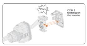
Figure 8-39 Inserting the connector to COM 1
