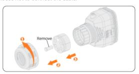
Figure 8-53 Disassembling the connector
