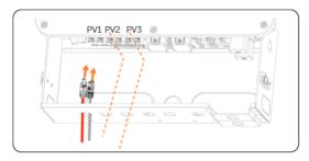
Figure 15-31 Connecting the PV cable
