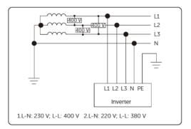
Figure 2-2 Supported power grid-TT
