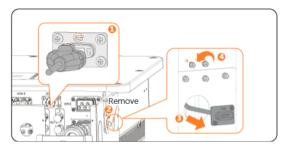
Figure 15-34 Installing the WiFi connecting cable
