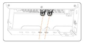
Figure 15-33 Connecting to COM port
