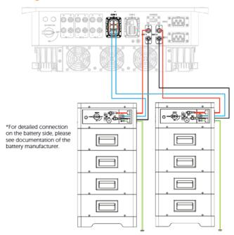
Figure 8-41 BMS connection diagram
