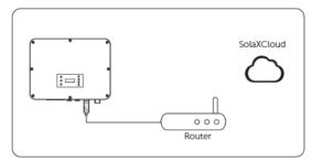
Figure 8-67 LAN mode connection diagram
