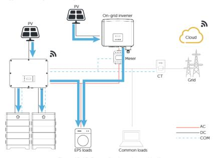
Figure 15-15 Power flowing when grid off
