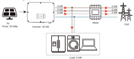
Figure 2-18 Zero export control with Phase Unbalance enabled
