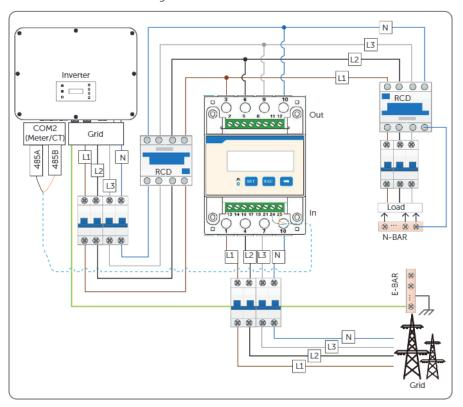
Figure 8-48 Meter connection diagram 1
