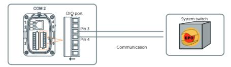
Figure 8-63 System switch connection diagram
