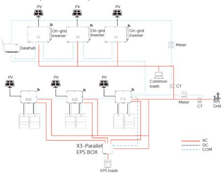
Figure 15-10 DataHub wiring diagram
