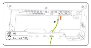
Figure 15-27 Connecting the PE cable
