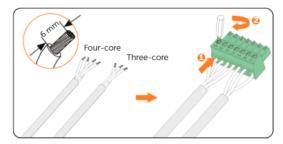
Figure 8-64 Connecting to 7-pin terminal block
