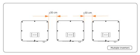
Figure 5-5 Clearance requirement for multiple inverter
