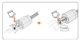
Figure 8-32 Press down on the Spring
