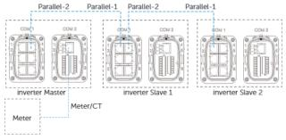
Figure 15-22 Communication connection without X3-PBOX
