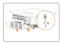
Figure 12-1 Disconnect the fans connectors
