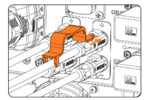
Figure 13-4 Removing the Battery connector
