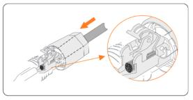
Figure 8-31 Threading the battery cable
