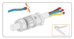
Figure 8-11 Striping the end of cable and crimping it
