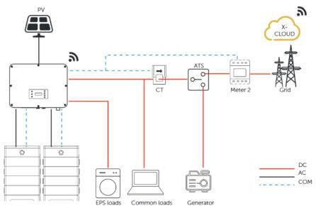
Figure 15-1 ATS control wiring diagram
