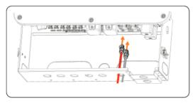
Figure 15-32 Connecting the battery power cable
