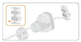
Figure 8-45 Installing RJ45 terminal to the cable fixture
