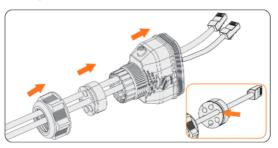
Figure 8-37 Threading the cables
