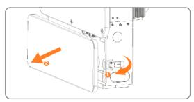
Figure 15-26 Removing the front panel
