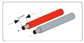
Figure 8-29 Striping the battery cable
