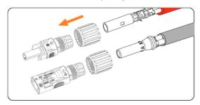
Figure 8-18 Threading the PV cable
