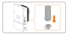
Figure 15-36 Installing the dongle
