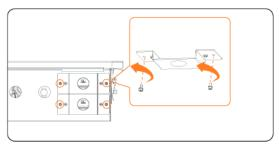
Figure 15-28 Loosening the screws from cable cover
