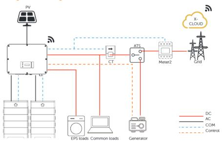
Figure 15-2 Dry contact wiring diagram
