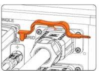
Figure 13-5 Removing AC connector
