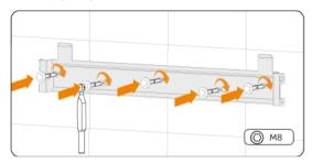
Figure 7-7 Inserting the screws
