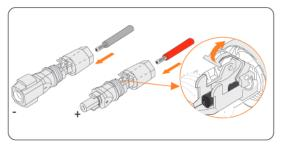
Figure 8-30 Opening the spring
