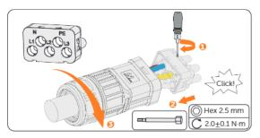
Figure 8-12 Assembling the AC connector
