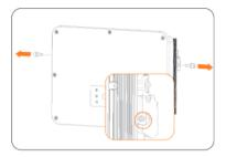
Figure 13-8 Unscrewing the M5 screws
