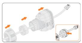
Figure 8-44 Threading the cables
