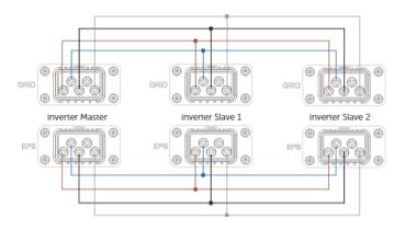
Figure 15-20 Power cable connection without X3-PBOX
