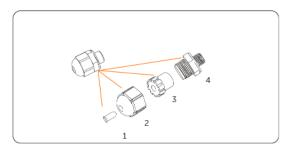
Figure 8-70 Disassembling the waterproof connector
