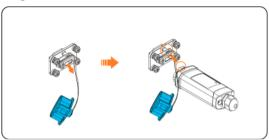
Figure 8-69 Wi-Fi connection procedure
