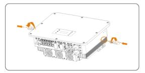
Figure 7-8 Installing the handles
