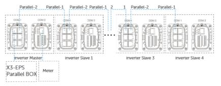
Figure 15-21 Communication connection with X3-PBOX
