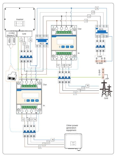
Figure 8-49 Meter connection diagram 2
