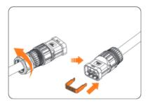
Figure 13-6 Remove the swivel nut
