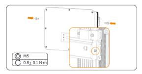
Figure 7-10 Securing the inverter
