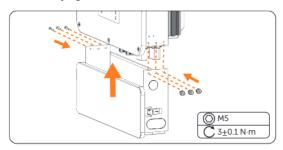
Figure 15-24 Installing the cable cover
