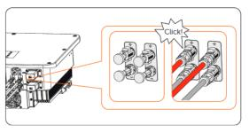
Figure 8-34 Connecting the battery connector
