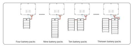
Figure 8-27 Battery connection Scheme 3
