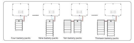
Figure 8-23 Battery connection Scheme 1
