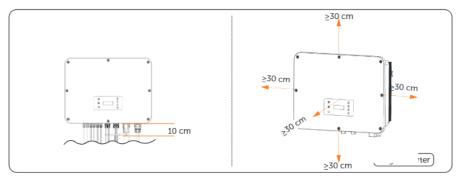
Figure 5-4 Clearance requirement for single inverter
