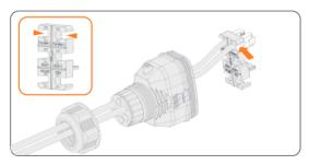
Figure 8-38 Installing RJ45 terminal to the cable fixture
