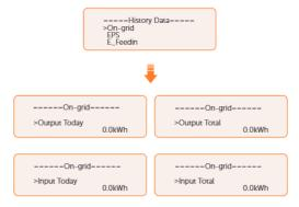
EPS: A record of the output electric energy of the inverter today and the total.
