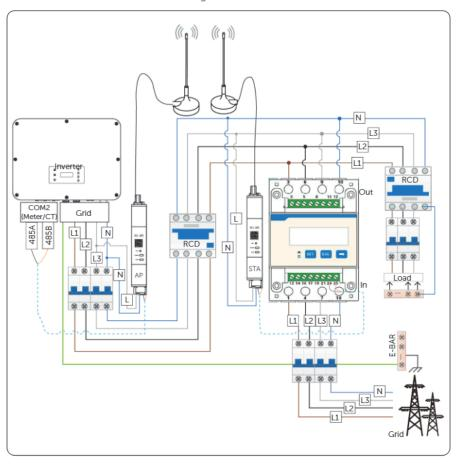
Figure 8-50 Wireless Meter connection diagram
