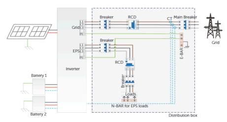
Figure 2-11 Application scheme for X3-ULT-10K / 15K-GLV
