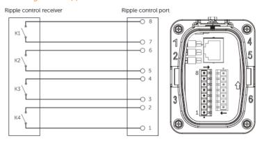
Figure 8-58 Connection diagram for ripple control
