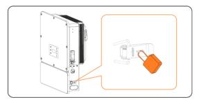
Figure 15-39 Installing the locks
