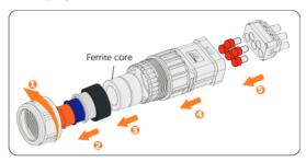
Figure 8-9 Disassembling the AC connector
