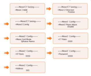
» Case 4: Meter 1 and Meter 2 are connected. (Meter 1 for SolaX Hybrid inverter, Meter 2 for another power generation equipment or Meter 1 for another power generation equipment, Meter 2 for SolaX Hybrid inverter). Please refer to Case 2 for Meter 1 setting and Case 3 for Meter 2 setting. You can check the connection status in Meter/CT Check.
