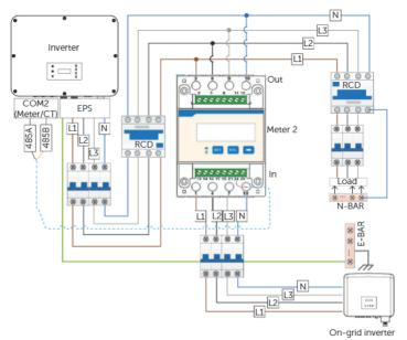
Figure 15-16 Connection diagram of Meter on EPS port
