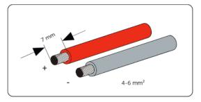
Figure 8-15 Striping the PV cable
