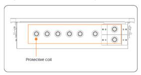
Figure 15-25 Removing the protective coil
