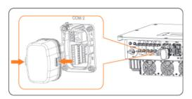
Figure 8-52 Disassembling the COM 2 port
