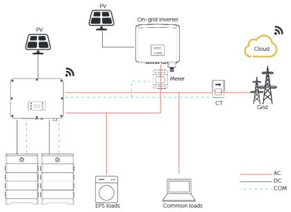
Figure 15-13 Micro-grid wiring connection
