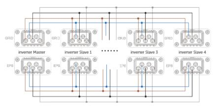
Figure 15-19 Power cable connection with X3-PBOX
