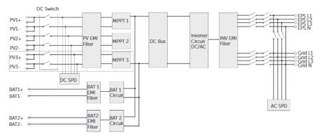
Figure 2-6 Circuit diagram for X3-ULTRA series inverter
