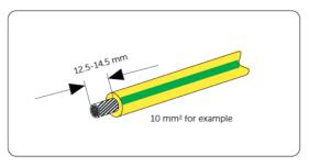
Figure 8-3 Striping the PE cable
