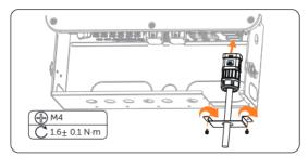
Figure 15-30 Installing the AC connector
