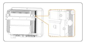
Figure 7-11 Locking the inverter
