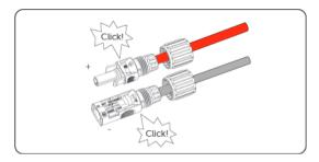
Figure 8-19 Securing the PV cable
