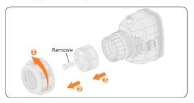
Figure 8-43 Disassembling the connector
