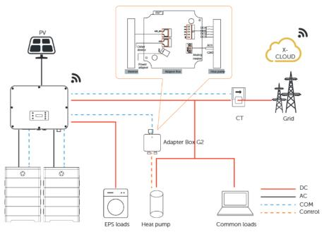
Figure 15-4 Adapter Box G2 wiring diagram
