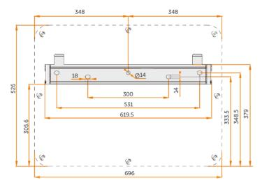
Figure 7-4 Dimensions 2 (Unit: mm)
