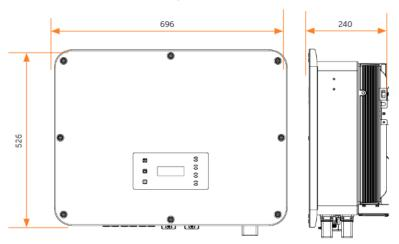
Figure 7-3 Dimensions 1 (Unit: mm)
