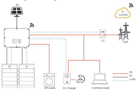
Figure 15-7 EV-Charger wiring diagram
