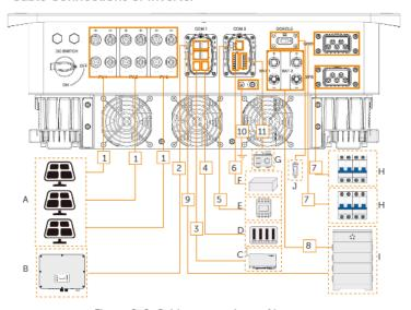
Figure 8-2 Cable connections of inverter
