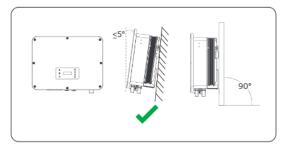
Figure 7-1 Correct installation
