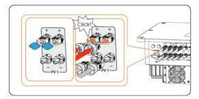
Figure 8-21 Connecting the PV cable
