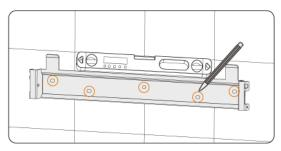
Figure 7-5 Marking the holes
