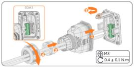
Figure 8-62 Connecting to the inverter
