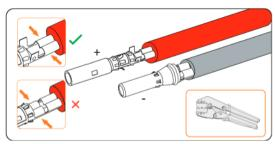
Figure 8-17 Crimping the terminal
