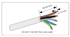
Figure 8-8 Stripping the Grid cable
