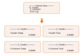
E\_USERDEF: The electricity of the connected on-grid inverter today and the total.(detected by Meter 2) This function is only available when the meter 2 is connected.
