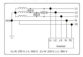
Figure 2-4 Supported power grid-TN-C-S
