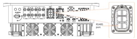
Figure 15-8 Connection port for EV-Charger
