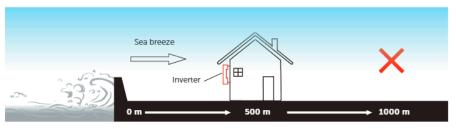
Figure 5-2 Incorrect installation position
