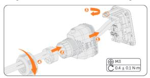
Figure 8-40 Securing the connector
