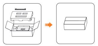
Figure 13-9 Packing the inverter
