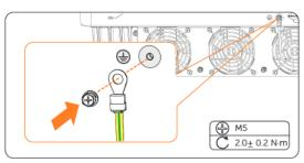
Figure 8-7 Securing the PE cable
