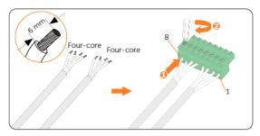
Figure 8-61 Connecting to 8-pin terminal block
