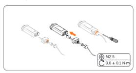
Figure 8-71 Assembling the dongle
