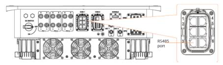
Figure 15-11 Connection port for DataHub
