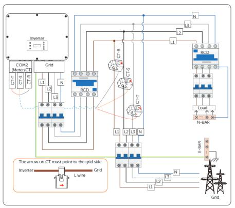
Figure 8-51 CT connection diagram
