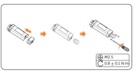
Figure 8-68 Assembling the dongle
