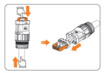
Figure 13-7 Disconnect the AC connector
