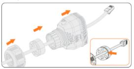
Figure 8-54 Threading the cables
