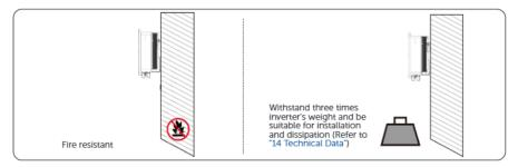
Figure 5-3 Installation carrier requirement
