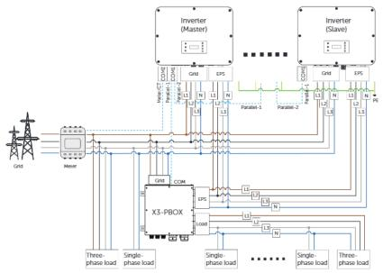
Figure 15-17 System diagram with SolaX X3-PBOX
