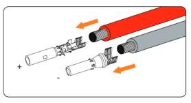
Figure 8-16 Inserting the PV pin contact
