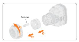
Figure 8-60 Disassembling the connector
