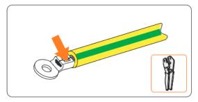
Figure 8-5 Crimping the cable
