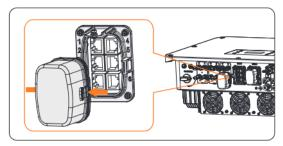
Figure 8-35 Removing the connector enclosure
