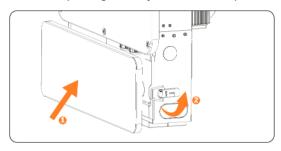
Figure 15-38 Installing the front panel
