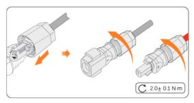
Figure 8-33 Tighten the cable gland
