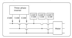
Figure 10-7 Phase Unbalanced enabled
