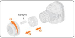
Figure 8-36 Disassembling the connector
