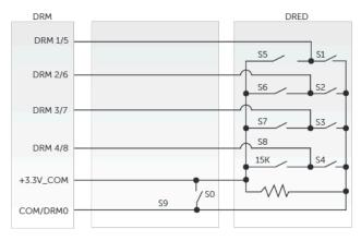
Figure 8-46 DRED wiring diagram
