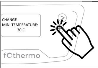
To change possible settings on an option page, such as the minimum temperature or the operating mode, briefly press the
