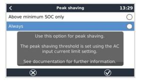
(Applies only when BatteryLife is enabled - it is always on in 'Keep batteries charged mode')
