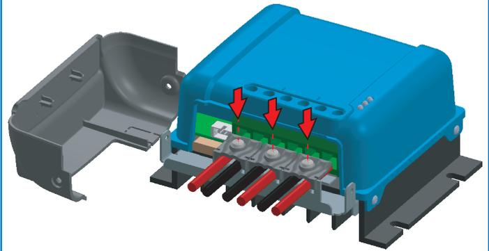
STEP 2: After mounting the MPPT to the wall, secure the cables (max Ø5 mm).
