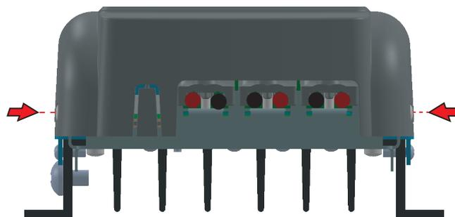
STEP 3: Place the WireBox cover and fasten with two screws.
