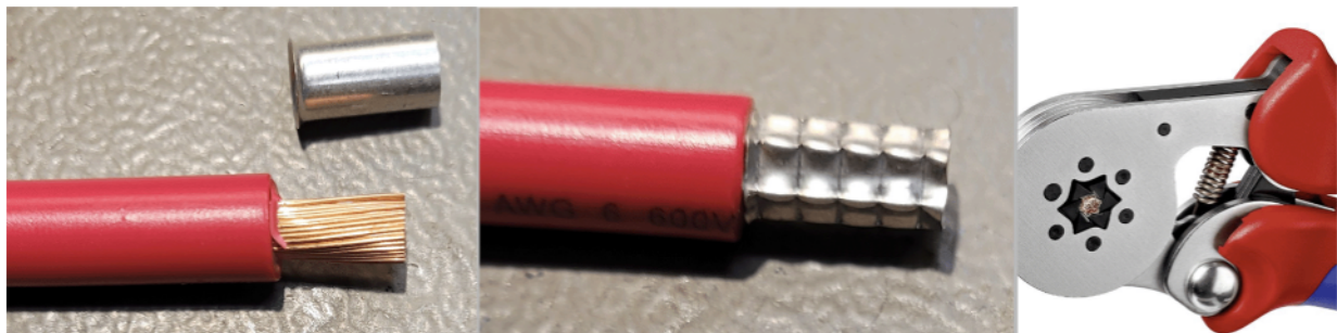
Hexagonally crimped bootlace ferrule
