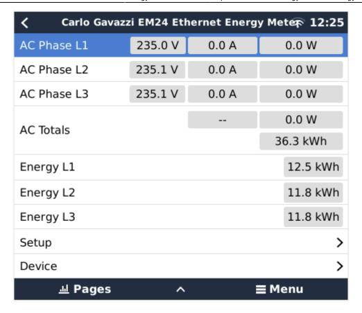
The role of the meter can also be changed through the Setup menu. The role will be one of Grid meter, PV inverter, or Generator.
