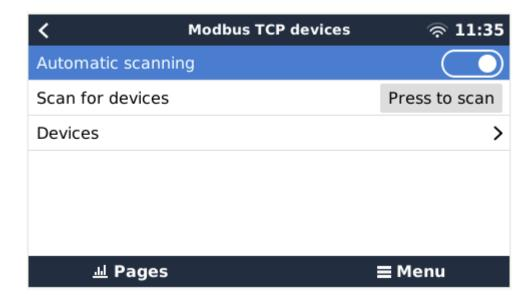
Once a meter is found, it will be shown under Devices. It is also possible to manually define the connection details of a meter, in case scanning does not locate it.
